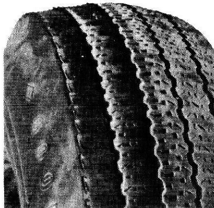
FEATHERING DUE TO MISALIGNMENT
