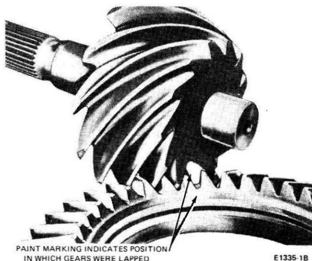
FIG. 32 Typical Gear Set Timing Marks
