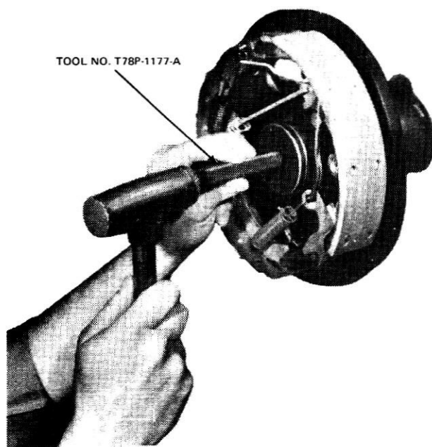
INSTALLATION OF WHEEL BEARING SEAL (1177)
