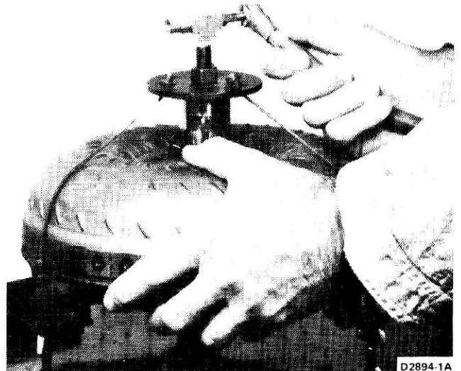
FIG. 4 Torque Converter Leak Detector Installed
