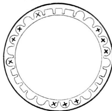
FIG. 42 Reverse-High Clutch Piston Return Spring Locations
