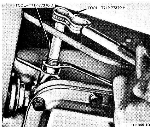
FIG. 9 Rear Band Adjustment—C4 Transmission
